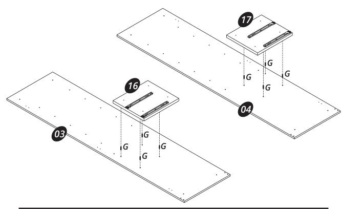
Mulberry side wardrobe Fix the hardware (H) onto the part (03) and the part (04) with the hardware (C). Connect the part (16) and part (17) with the hardware (D).
